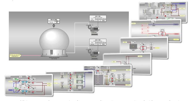
In addition to complete operational access, scada stations are equipped with comprehensive trends and history. Local HMI displays have access to alarm lists, but not to process history and trends. Scada stations can operate on one or two monitors, and they are equal in operational hierarchy. Even so, stations are configured as server and client. For client station to be fully operational, server station must be online and running.
